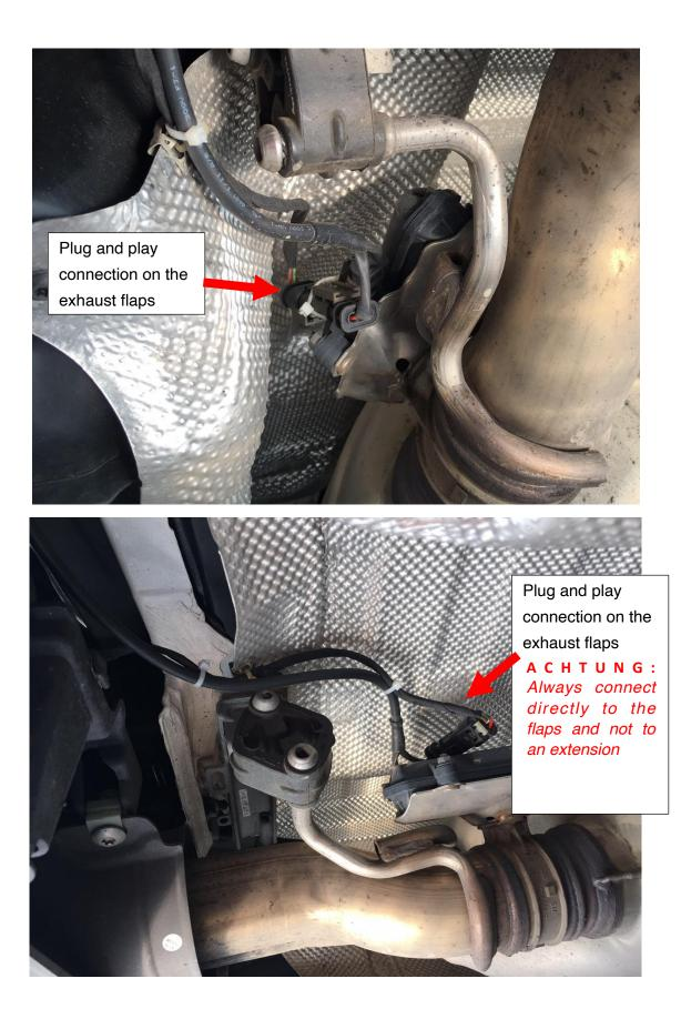
Disconnect the wire harness at the valve motor body and insert the ASR harness at this point. DO NOT connect to the extension cable to prevent errors and loss of power. If in doubt please watch the video
